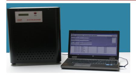
The DATAGONE LG is a fully automatic degausser for Hard Disks and Backup tapes with a unique Erasure Log Software. It uses pulse discharge technology and is fully processor controlled which enables the DATAGONE to offer a complete and secure erase on magnetic media.
